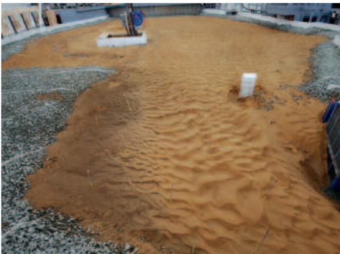
Figure 2 - Comprehensive mobile-bed model using low-density model sediments
