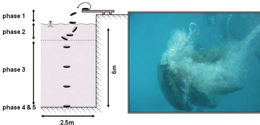
Fig. 12. Schematic of sinking behavior of dumped geotextile bags, and photo of dropped heap of three bags during the initial sinking process (Zellweger, 2007).
