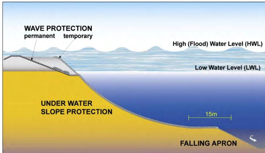
Fig. 13. The three elements of geotextile bag revetments.
