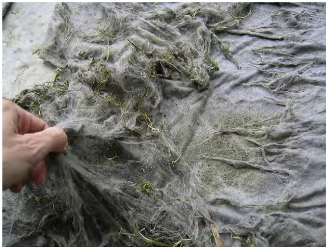
**Fig. 1.** A geotextile bag from the wave zone at the Bahadurabad test site on the Jamuna River. The bond between the fibers is destroyed and the bag is open. The bag was placed in early 1997, and the photo was taken in early 2005.
