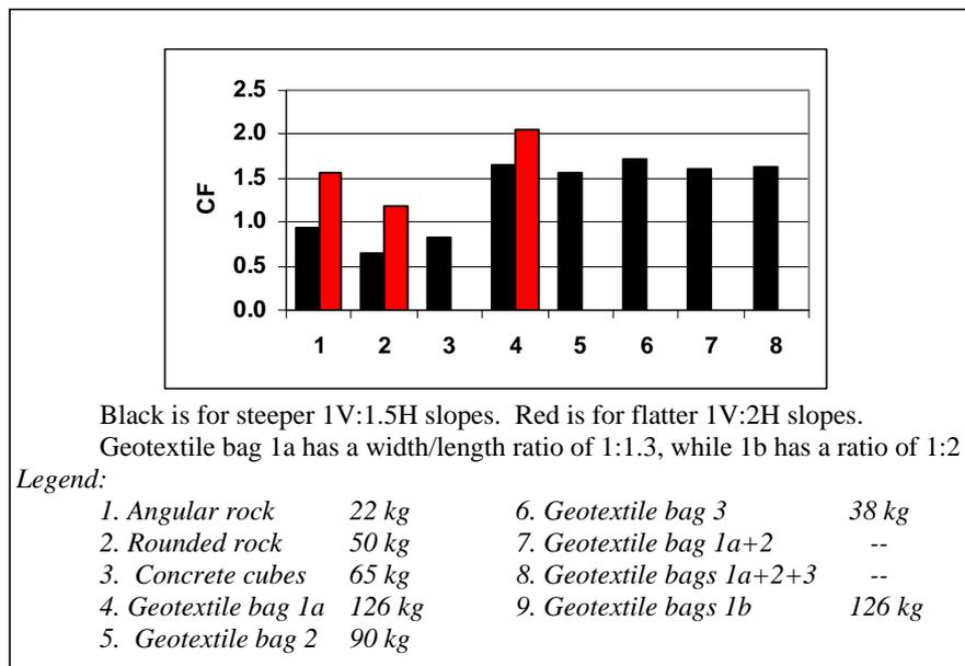
Fig. 10. C.F. coefficient required for displacement of protective elements on slopes (Stevens and Oberhagemann, 2006).
