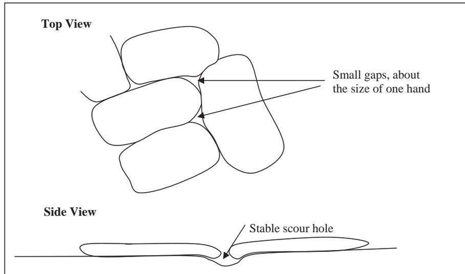
Fig. 7. Single coverage with geotextile bags, leaving small stable holes in the underlying sand.
