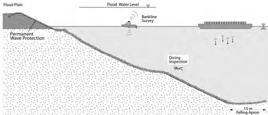
Fig. 16. Adaptive protection through dumping to greater depths.
