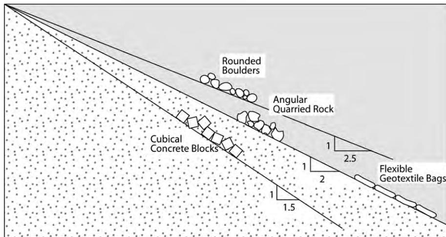
Fig. 5. Launching slopes of different protective materials (JMREMP, 2006).
