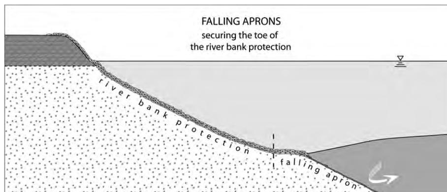
Fig. 4. The principle of falling aprons to protect against future scour (dark grey).
