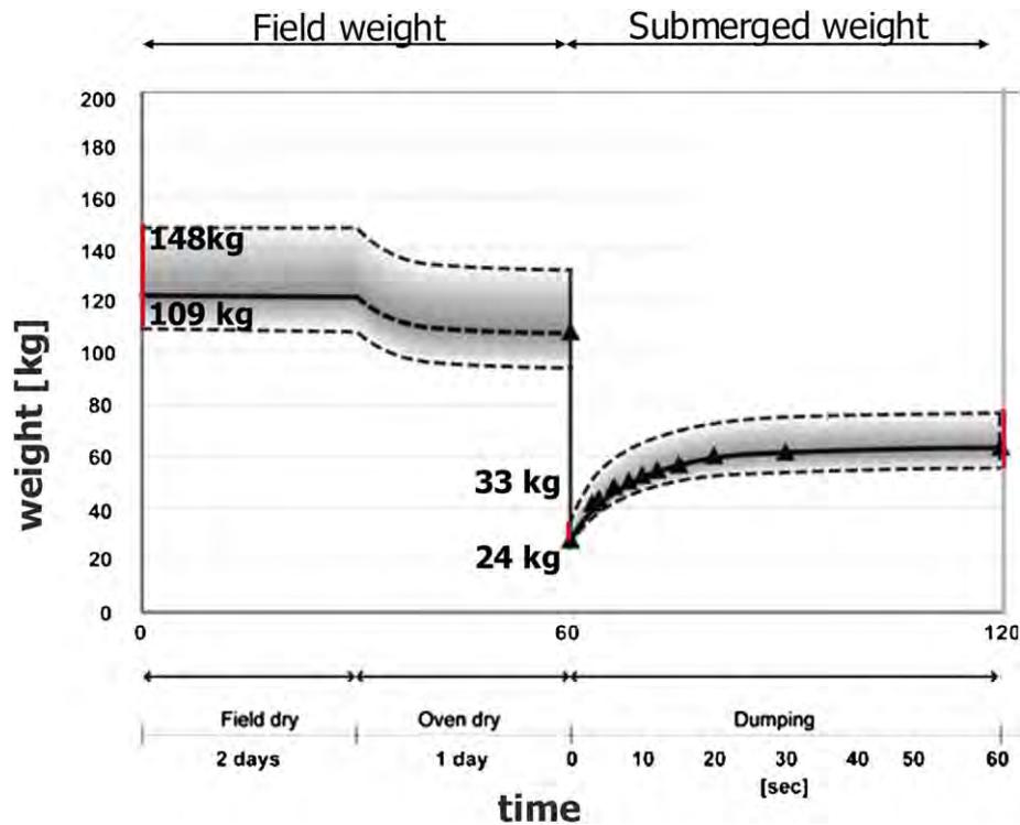
Fig. 11. Development of initial submerged weight depending on the moisture content of the sand fill (Zellweger, 2007).
