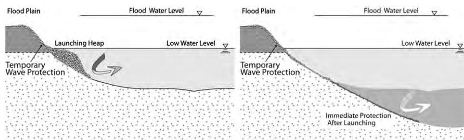
Fig. 14. Emergency protection through mass dumping of a launching heap along the bank.
