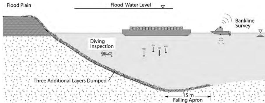
Fig. 15. Main protection through dumping of additional layers.
